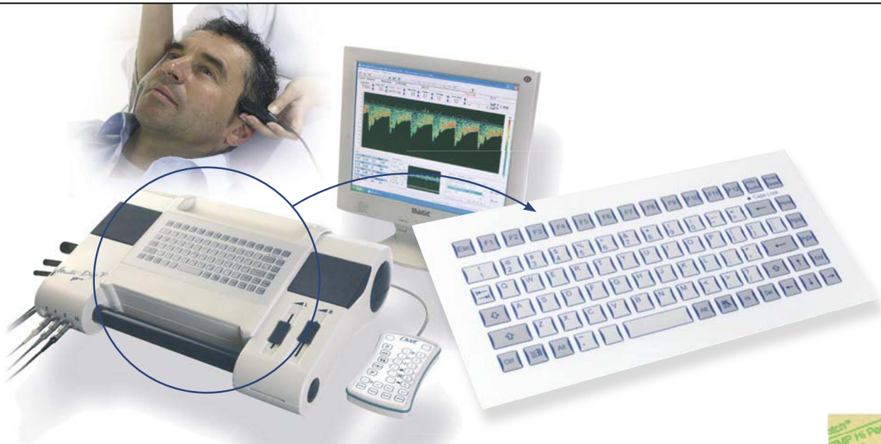
A dome switch keyboard in a blood pressure device
